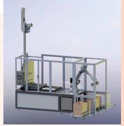
In this area, the "Comau" robot equipped with a gripping hand picks up the rows and places them in an orderly manner inside a carton box, which is manually opened and positioned on a motorized system that advances the boxes, placing them in the loading area when requested.
